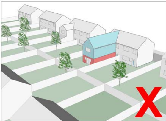
The extension's size dominates & it fails to meet the 45° & 60° rule
