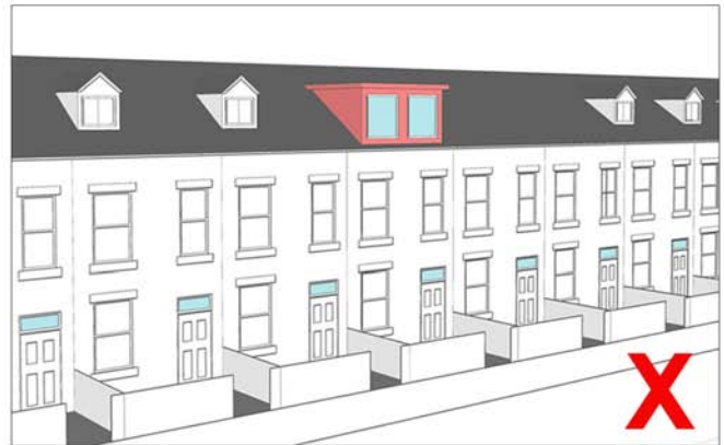
Flat roofed, exceeds 1/3 of roof space & fails to acknowledge surroundings
