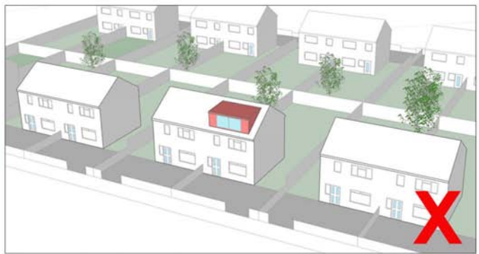
Dominates the roof space, has a flat roof & detracts from surrounding character
