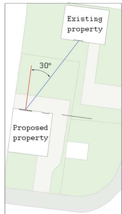
C. Measure the angle between the two lines to gain (X) for the equation
