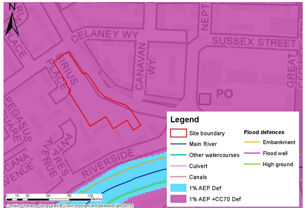
Figure 4: Defended fluvial outlines for the present day 1% AEP and future risk 1% AEP with +70% AEP climate change uplift.
