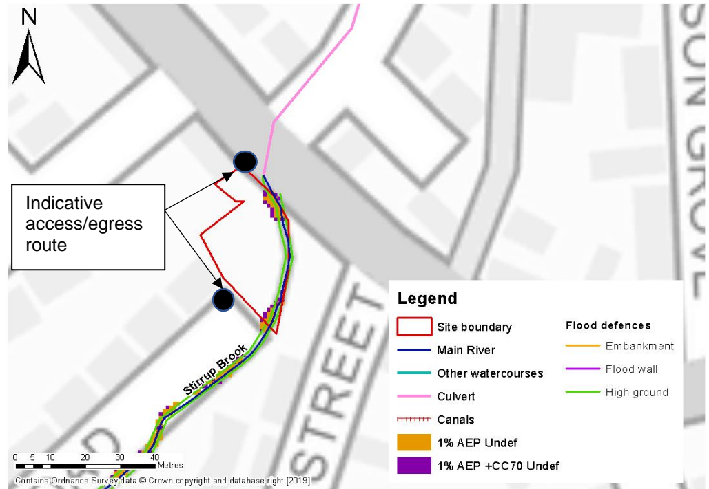
Figure 2: Undefended fluvial outlines for the present day 1% AEP and future risk 1% AEP with +70% climate change uplift
