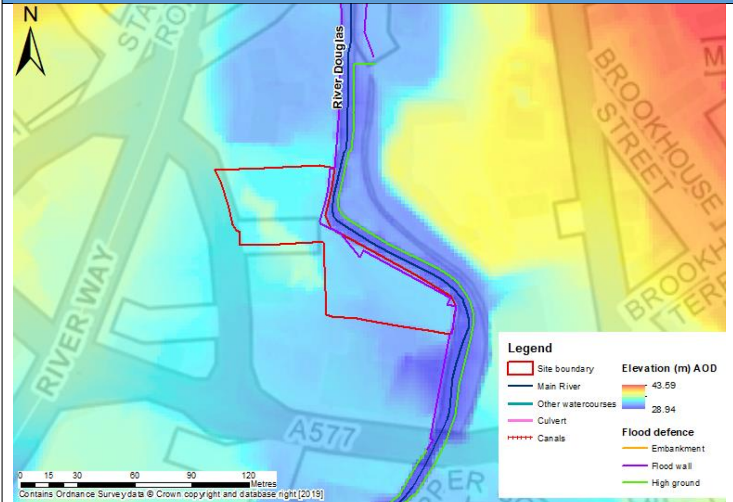
Figure 2: Site with 2 m 2017 LIDAR (elevation data)
