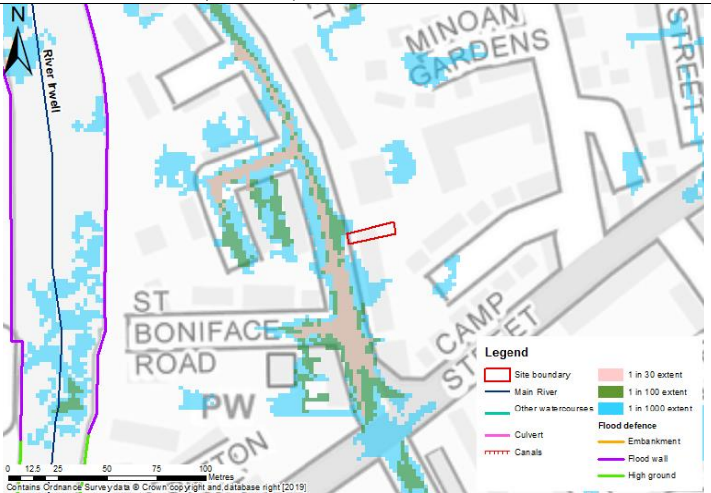
Figure 4: Surface water risk to the site (Risk of Flooding from Surface Water map)
